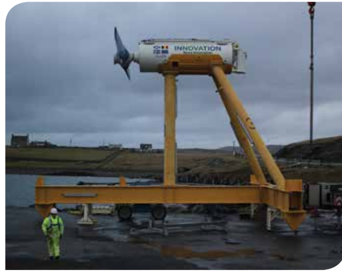
A tidal generator ready to be installed as part of the NiNES ANM scheme in Shetland.
